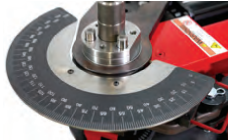
Large, easy to read degree dial for accurate bends
