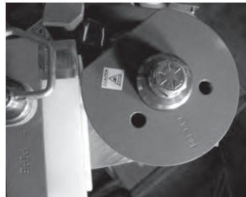
Figure 8.6 - Correct: Approximately 1/8" (3mm) Away
