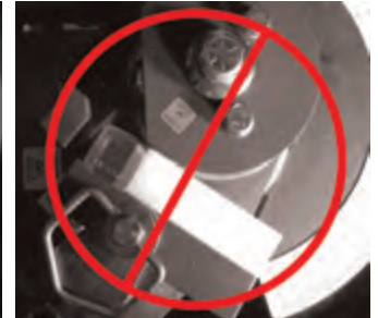
Figure 8.5 - Incorrect: Touching Die
